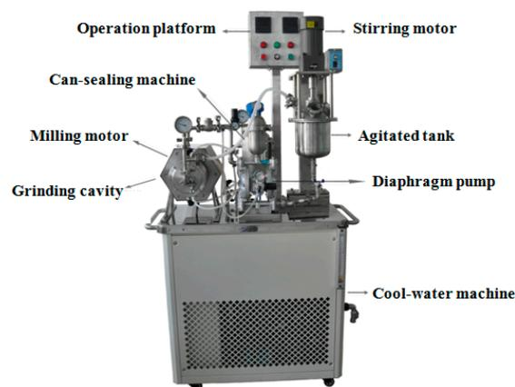
**Figure 1.** Image of the nano sand-mill.
