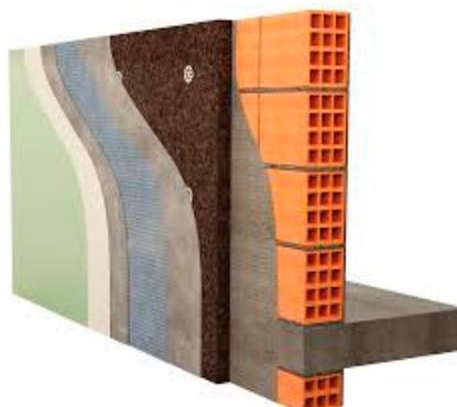
**Figure 1.** Insulation cork board (ICB) in an External Thermal Insulation Composite System (ETICS) [9].
