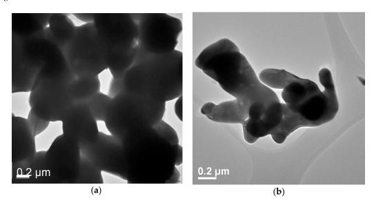
**Figure S2.** TEM images of particles scraped from WO<sub>3</sub>/CuWO<sub>4</sub>, indicating network morphology of the CuWO<sub>4</sub> layer. (**a**) Network structure of CuWO<sub>4</sub> layer; (**b**) Branched CuWO<sub>4</sub> nanoparticles from broken network piece.
