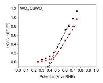
**Figure S4.** Mott-Schottky plots of WO<sub>3</sub>/CuWO<sub>4</sub> thin film at 10 k (black) and 5 k Hz (red) under dark condition.
