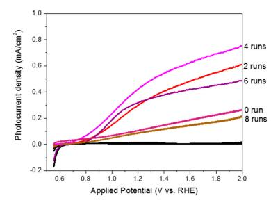
**Figure S3.** Photocurrent comparison of thin film obtained from different runs of dip coating. (Colored lines: Photocurrent under AM 1.5G illumination, Black lines: dark current).
