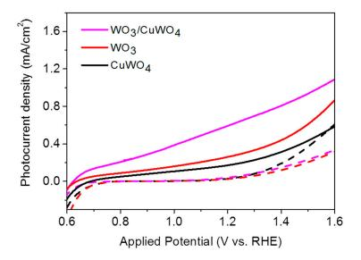
**Figure S6.** Linear sweep voltammetry of all samples with (solid lines) and without the illumination of AM 1.5 (dashed lines), measured in 0.5 M Na<sub>2</sub>SO<sub>4</sub> + 0.5 M H<sub>2</sub>O<sub>2</sub> aqueous solution.
