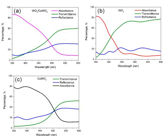
**Figure S5.** Absorption efficiency of: (a) WO<sub>3</sub>/CuWO<sub>4</sub>; (b) WO<sub>3</sub>; and (c) CuWO<sub>4</sub> thin films by measuring the transmission and reflection spectra using an integrating sphere (Absorbance ( $\eta_{abs}$ ) = 1 – Transmittance – Reflectance).
