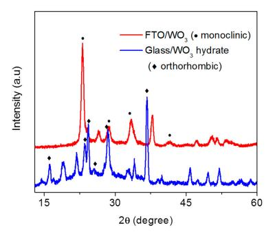
**Figure S1.** XRD patterns of different WO<sub>3</sub> phases obtained from magnetron sputtering on FTO (**red**) and normal glass slide (**blue**) substrates, which showed the FTO layer helped to induce the crystal growth of monoclinic WO<sub>3</sub>.
