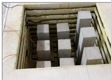
Figure 6. Samples in furnace.
