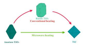
Figure 1. Schematic of different reaction routes between conventional and microwave heating.
