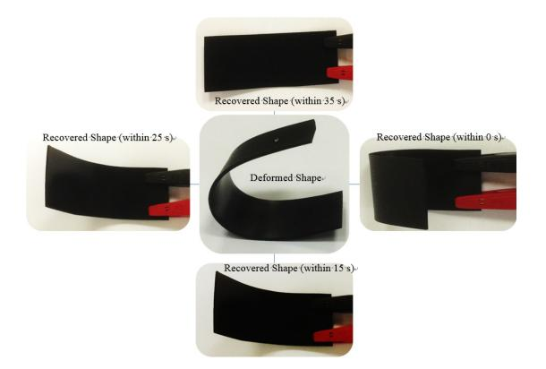
Figure 3. Electroactive shape recovery behaviour of the Cu-CNT dispersed PLA/ESO nanocomposite (Cu-CNTs content of 2 wt %) at a DC voltage of 40 V.
