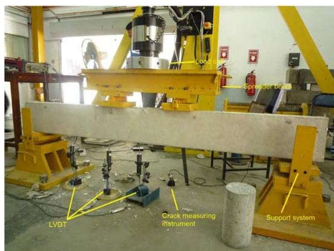
**Figure 8.** Experimental setup.
