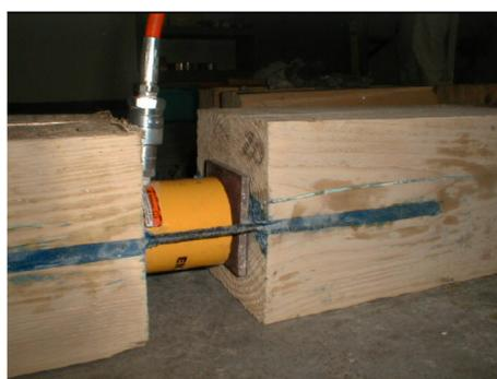
**Figure 7.** Pull-out test arrangement (tests without strain gauges).
