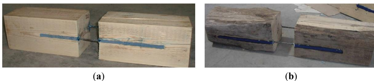
**Figure 5.** (a) Fir wood specimen; (b) chestnut wood specimen.
