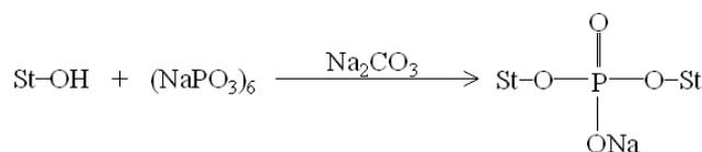
**Scheme 1.** Reaction mechanism of sodium hexametaphosphate and starch molecules [47].
