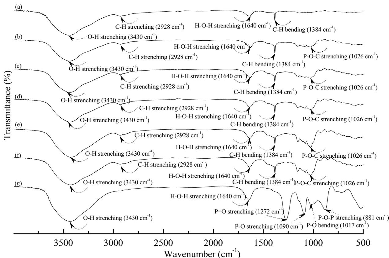
**Figure 1.** FTIR spectra of (a)  $\text{TPS}_{100}\text{BC}_{0.02}$ ; (b)  $\text{TPS}_{100}\text{BC}_{0.02}\text{SHMP}_4$ ; (c)  $\text{TPS}_{100}\text{BC}_{0.02}\text{SHMP}_8$ ; (d)  $\text{TPS}_{100}\text{BC}_{0.02}\text{SHMP}_{10}$ ; (e)  $\text{TPS}_{100}\text{BC}_{0.02}\text{SHMP}_{16}$ ; (f)  $\text{TPS}_{100}\text{BC}_{0.02}\text{SHMP}_{32}$  and (g) SHMP specimens.
