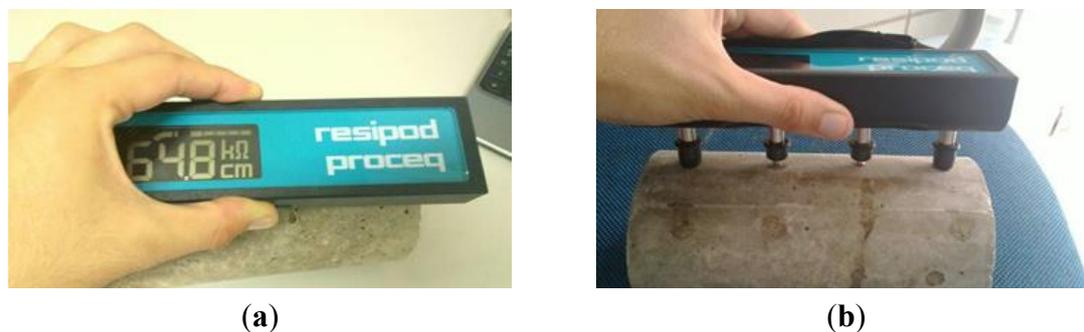
**Figure 4.** Visualization and measurement of the electrical resistivity. (a) electrical resistivity apparatus; (b) measuring electrical resistivity.
