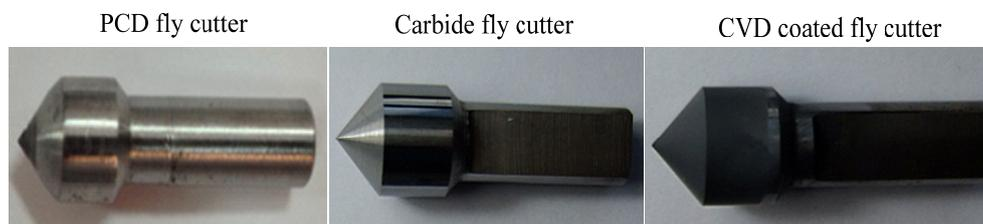
**Figure 2.** Cutting tools in experiments.
