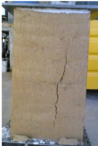
Figure 9. A specimen (40 \times 40 \times 70) \text{ cm}^3 after the compression test.
