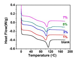
Figure 1. DSC thermograms of xLCNs/SiO<sub>2</sub> composites (xLCN/SNP) and blank xLCN.
