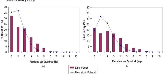
Figure 20. Particle distribution of SiC particles in Zn-Al matrix (a) heat treated; (b) 35% cold rolled [104].
