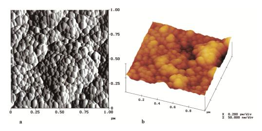
**Figure 15.** TEM micrograph of the  $Al_2O_3$  nanocomposite thin film reinforced with NdAlO<sub>3</sub> nanocrystallites, deposited on a Si target by CVD and sintered at 1400 °C [44].
