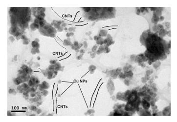
**Figure 4.** HRTEM micrograph of as-consolidated CNT reinforced Cu matrix nanocomposite fabricated via molecular level mixing and vacuum sintering technologies [34].
