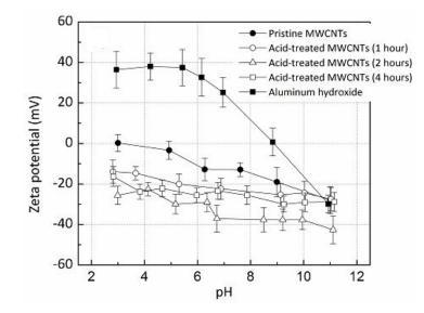
Figure 17. Zeta potential values of MWCNTs and acid-treated MWCNTs at different pH [9].
