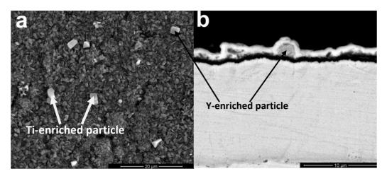
**Figure 5.** XRD Elemental mapping of the Y-enriched particle formed on the K38-0.5Y coating surface at 900 °C.
