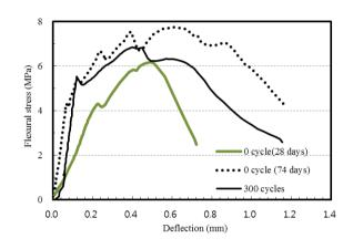
Figure 6. Typical flexural responses of 2SHCC prisms.
