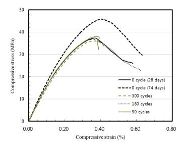
Figure 4. Typical compressive stress-strain curves of 2SHCC cylinders.
