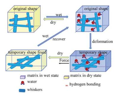
The combination of a percolation network of cellulose whiskers and an elastomer matrix is the microstructural prerequisite for the rapidly switchable water-sensitive shape-memory effect in these
