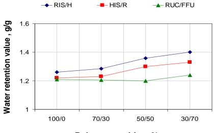
Figure 3. Water retention value (WRV) in relation with pulp composition.
