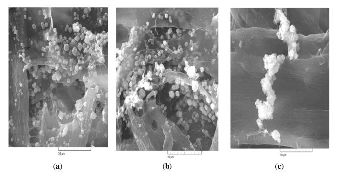
SEM images show that between the two types of pulp with *in-situ* loading (RIS and HIS) there are no significant differences regarding the calcium carbonate contents, but values of air permeability (Figure 6) show significant structural differences.
