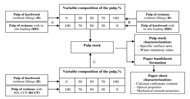
Figure 1. Experimental program for the three series of pulp with different composition.
