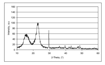
Figure 7. X-ray diffraction patterns of paper samples obtained by *in-situ* loading method.
