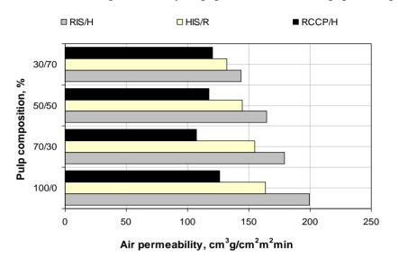
Figure 6. Evolution of air permeability of paper in relation with paper composition.
