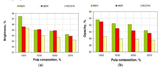
**Figure 9.** Evolution of properties in relation with pulp composition (**a**) brightness and (**b**) opacity.
