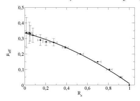
We see that as  $\mu_{eff}$  increases, the value of the sliding ratio s R decreases. The effective friction coefficient is saturated at a value equal to 0.33 for a sliding ratio equal to 0 (*i.e.*, a rolling without sliding state). This corresponds indeed to the value of the saturation observed on the previous curve (Figure 8). This saturated value of the effective friction coefficient depends essentially on certain
