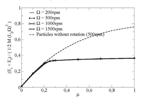
In this figure, we observe also the transition from a sliding regime towards a rolling without sliding regime. We note a saturation of the sum of the energy from a critical value of the friction coefficient, this satured value being independent of the rotational velocity of the vane.
