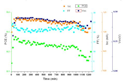
In contrast, cells from the gradient experiments on the R2R process had a T80 < 30 minutes dominated by a decrease in open circuit voltage. Modules made on the R2R process were observed to
