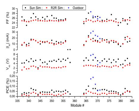
Furthermore, the use of an R2R simulator, an AM1.5G sun simulator and outdoor testing showed a significant difference between the performances of the modules. On the R2R simulator the  $V_{oc}$  was generally lower than what was measured later on the stationary sun simulator. Interestingly, the outdoor measurements showed even greater performance with the four outdoor modules showing an increase in PCE to almost double of the indoor measurement for the modules without extra
