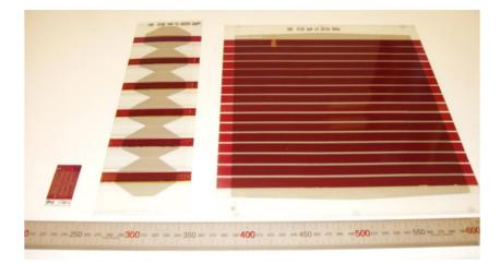
**Figure 3.** Image of a typical glass cell, gradient cell, and 16 cell module (from left to right) with a mm scale.
