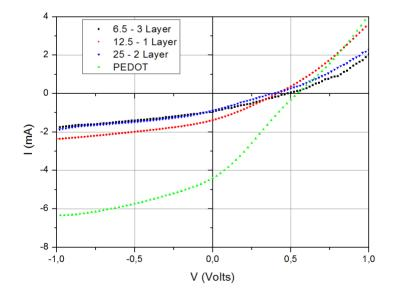
These initial test results indicated that there is a range of concentration between 6.5 and 25 mg/mL for which the cells have an acceptable performance for spin coated films on glass substrates. It is clear
