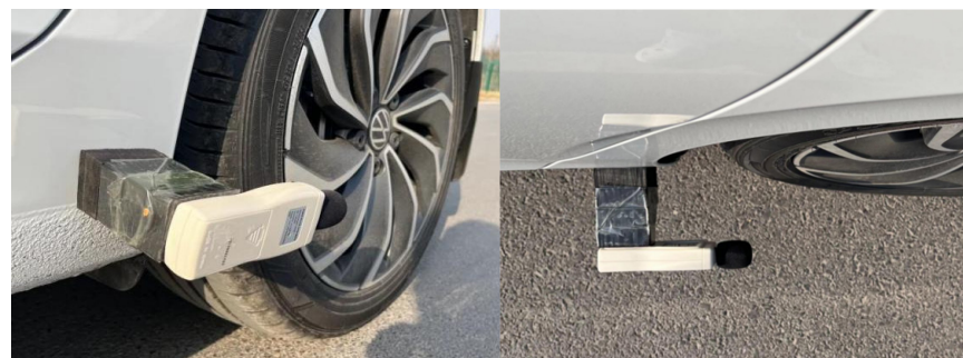
Figure 1. Near-field noise test noise meter layout.
