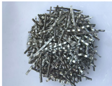
Shear steel fiber with an aspect ratio of 50.
