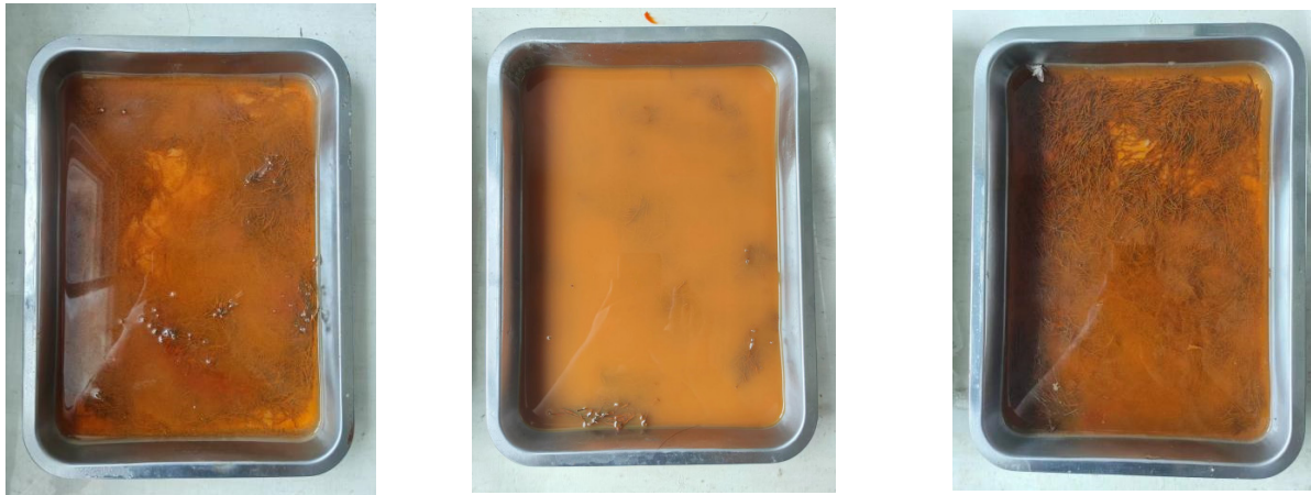
Soaked in 5% NaCl solution for 7 days. Soaked in 10% NaCl solution for 7 days. Soaked in 15% NaCl solution for 7 days.
