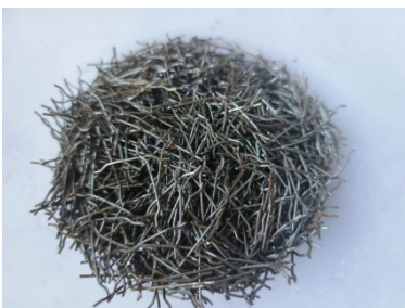
End-hook steel fiber with a length–diameter ratio of 40.
