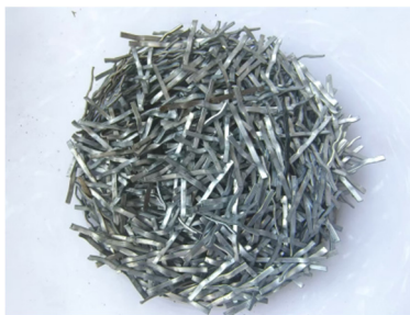
Milling steel fiber with an aspect ratio of 40.
