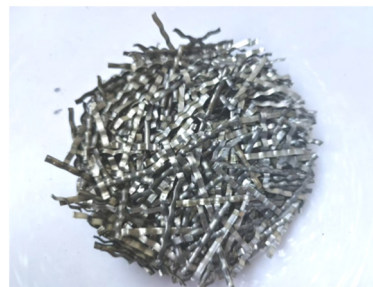
Milling steel fiber with an aspect ratio of 50.
