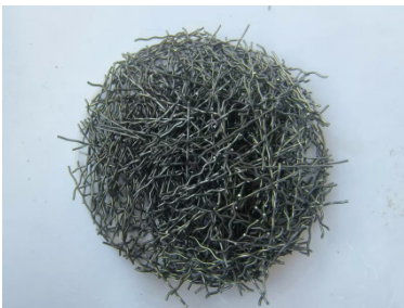
Shear steel fiber with an aspect ratio of 40.
