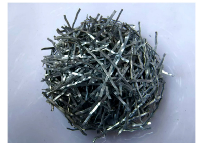
Shear steel fiber with an aspect ratio of 60.
