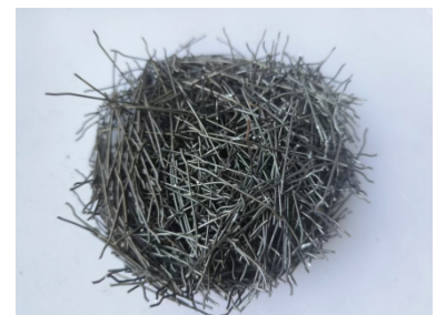
End-hook steel fiber with a length–diameter ratio of 60.
