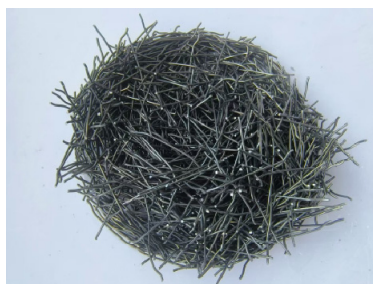
End-hook steel fiber with a length–diameter ratio of 50.
