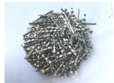
Milling steel fiber with an aspect ratio of 60.
