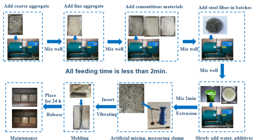
Figure 7. Flow chart of steel fiber cement concrete mixing.
