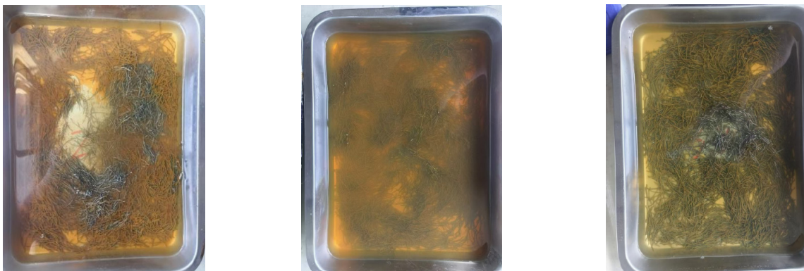
Soaked in 5% NaCl solution for 3 days. Soaked in 10% NaCl solution for 3 days. Soaked in 15% NaCl solution for 3 days.
