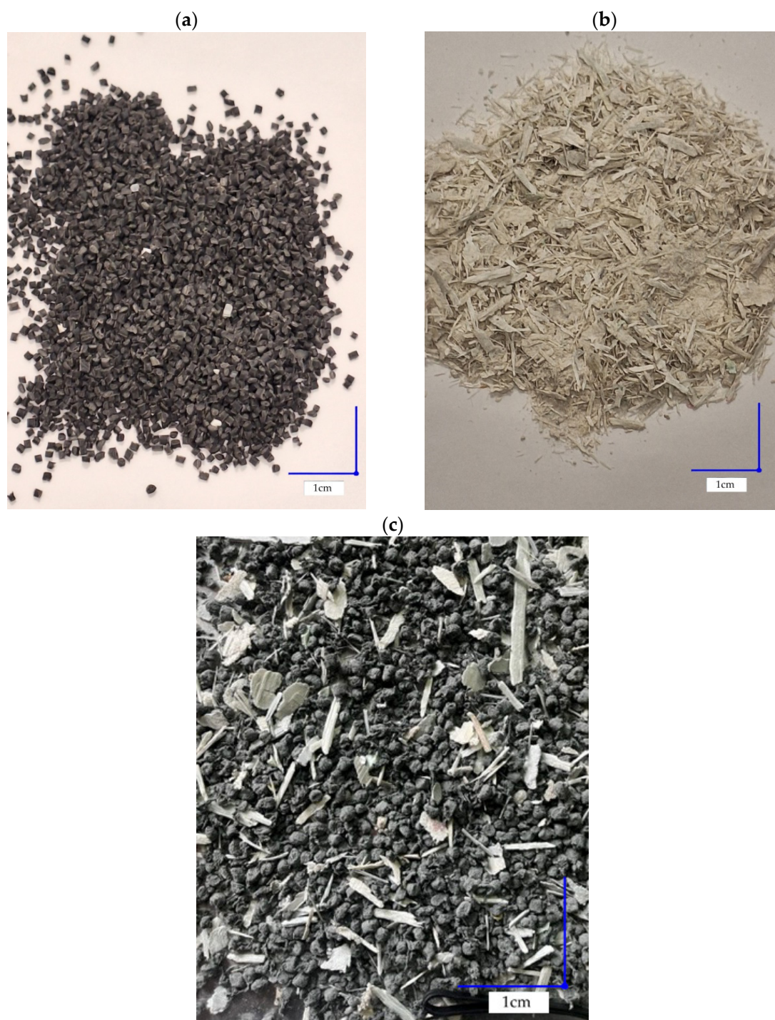
Figure 2. Raw materials used for composite plate fabrication: (a) reggranulate obtained from mechanically recycled post-consumer textile waste, (b) ground GFRP fraction derived from decommissioned wind turbine blades, (c) example of the mixed composite feedstock prior to pressing.
