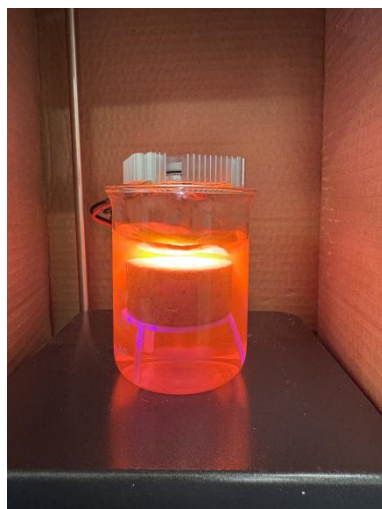
Figure 2. Photocatalytic performance testing setup of cement mortar-based catalysts.
