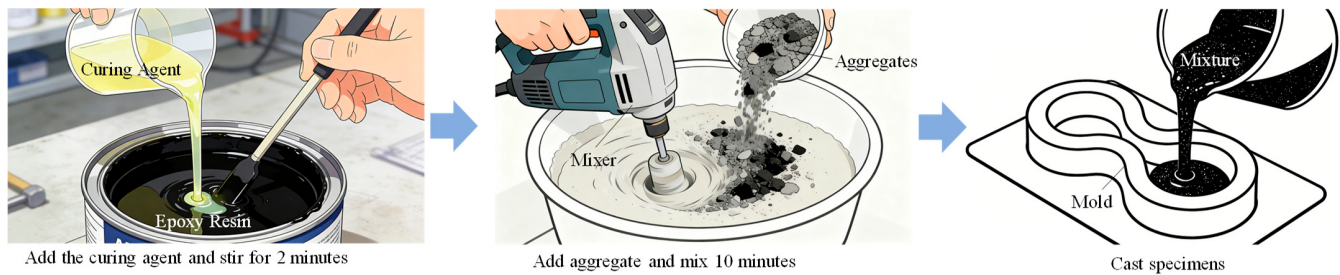
Figure 1. Schematic diagram of ERC specimen preparation.
