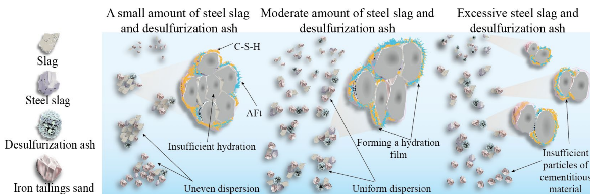
Figure 16. Analysis of the rheological characteristic mechanism of SW slurry.
