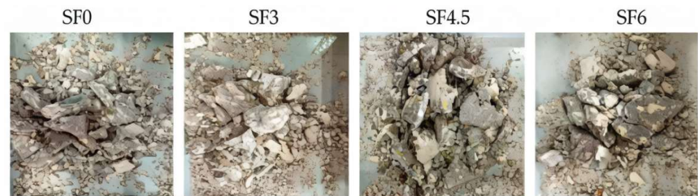
Figure 16. Impact compression failure diagram [85].
