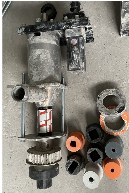
Figure 6. 3DCP printhead with various orifice sizes and geometries (round 10, 15 mm, rectangular 20 by 40 mm, square 20 and 30 mm). Courtesy of ATMAT.
