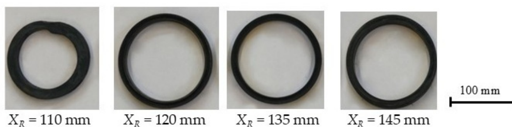
Figure 8. Selected rings obtained during the process carried out with a feed rate of 5 mm/s.
