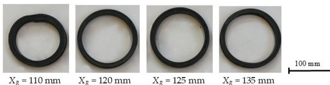
Figure 7. Selected rings obtained during the process carried out with a feed rate of 20 mm/s.
