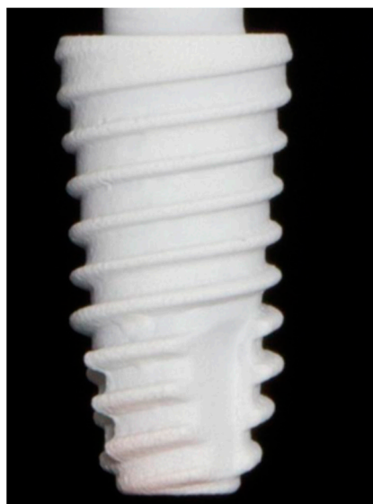
Figure 9. BG coating on a titanium implant screw via electrophoretic deposition [140]. (Adapted from https://creativecommons.org/licenses/by/4.0/ (accessed on 1 November 2025)).
