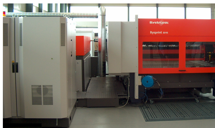
Figure 2. Laser cutting device used for samples cutting process.
