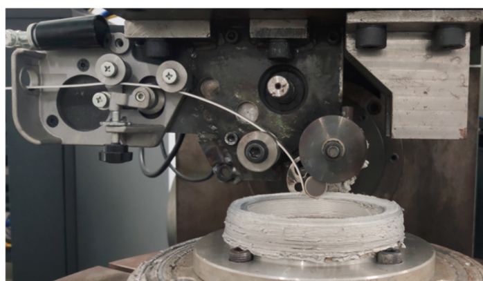
Figure 1. Experimental procedure for the fabrication of ring shape components using FRAM.
