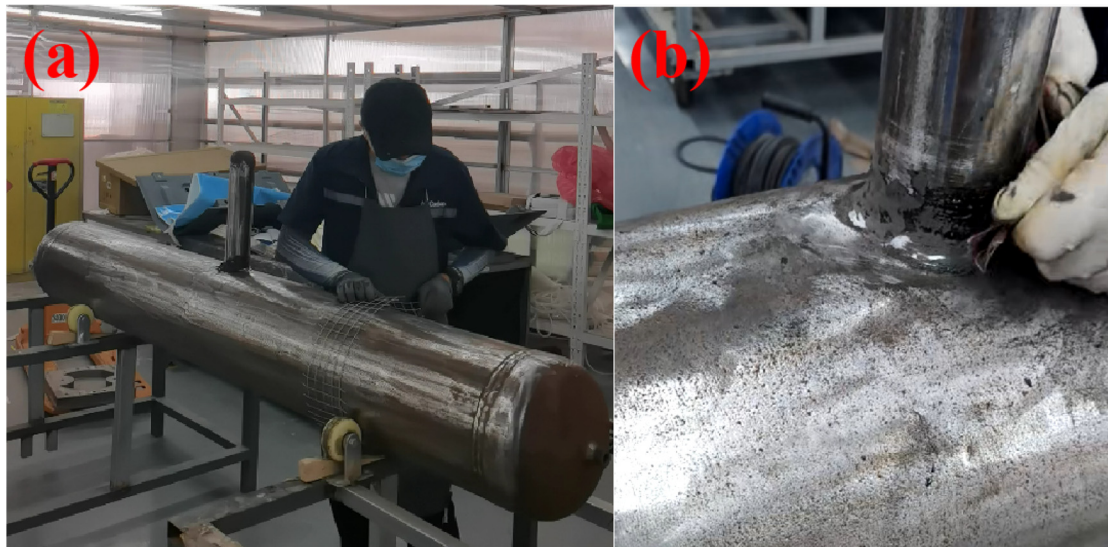
Figure 4. (a) Schematic diagram of winding fixture setting; (b) Schematic diagram of surface filling treatment for weld seam.
