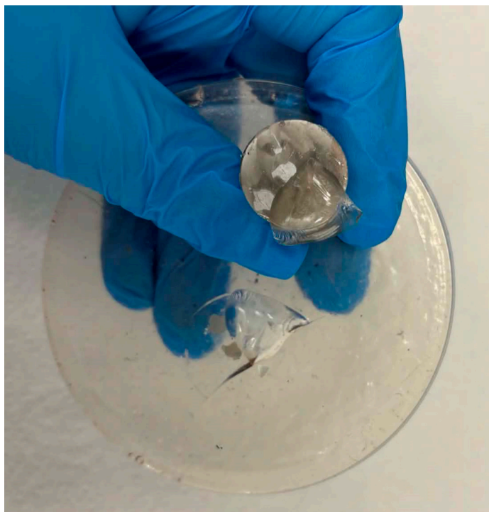
Figure 8. Representative cohesive failure of the Cl_0.5 composite after pull-off testing. The aluminium dolly detached together with a fragment of the composite material.
