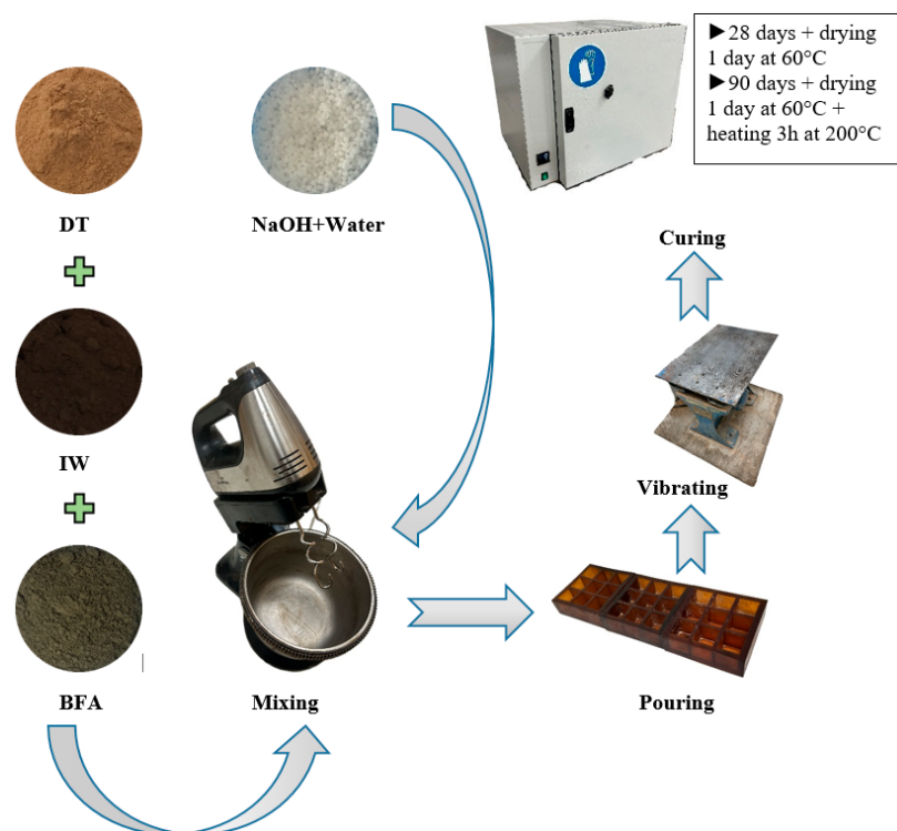
Figure 6. Order of the sample preparation steps. The arrow \Rightarrow indicates the order in the preparation of the samples. The arrow \blacktriangleright refers to the curing conditions for the test samples.
