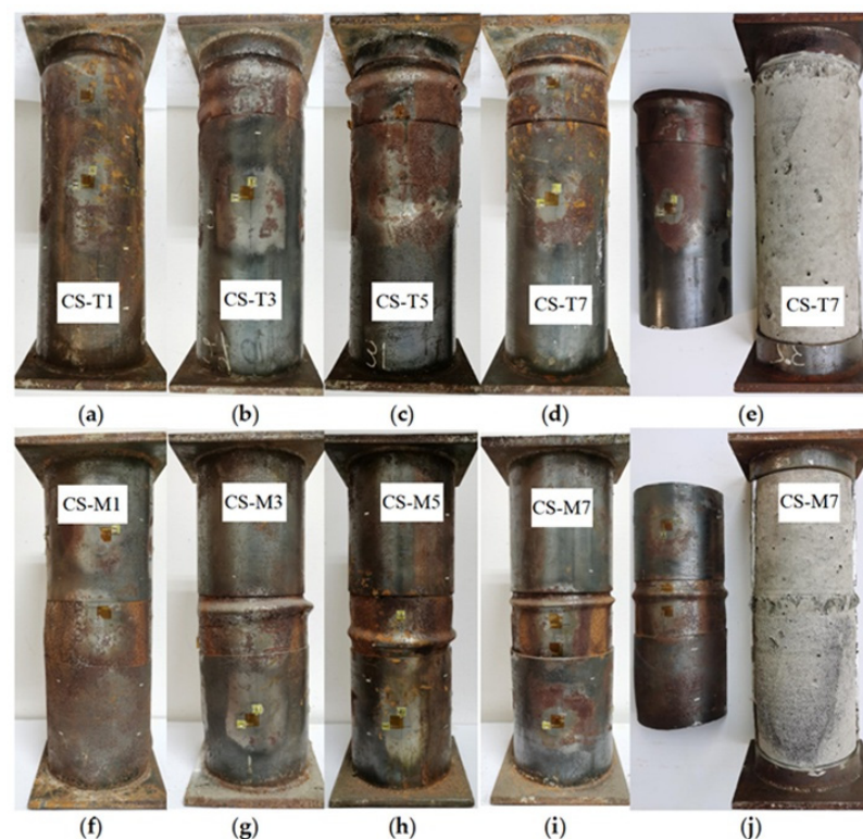
Figure 7. Failure patterns of CFST columns [64]: Failure modes of locally corroded CFST columns after axial compression tests: (a) CS-T1 (top corrosion, 10%); (b) CS-T3 (top corrosion, 30%); (c) CS-T5 (top corrosion, 50%); (d) CS-T7 (top corrosion, 70%); (e) separated steel tube and concrete core of CS-T7; (f) CS-M1 (mid-height corrosion, 10%); (g) CS-M3 (mid-height corrosion, 30%); (h) CS-M5 (mid-height corrosion, 50%); (i) CS-M7 (mid-height corrosion, 70%); (j) separated steel tube and concrete core of CS-M7.
