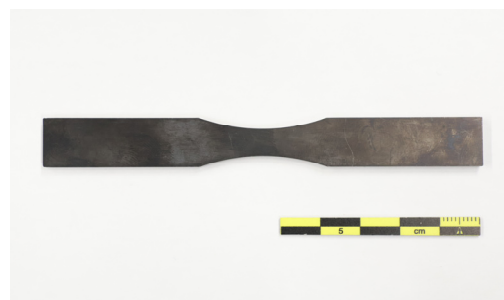
Figure 6. Sample after oxidation.
