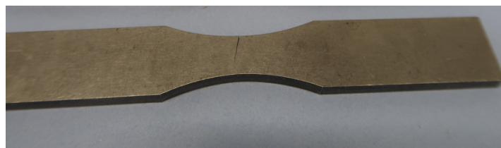
Figure 17. Hardened and tempered sample after fatigue test.
