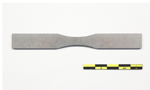
Figure 5. Sample before oxidation.
