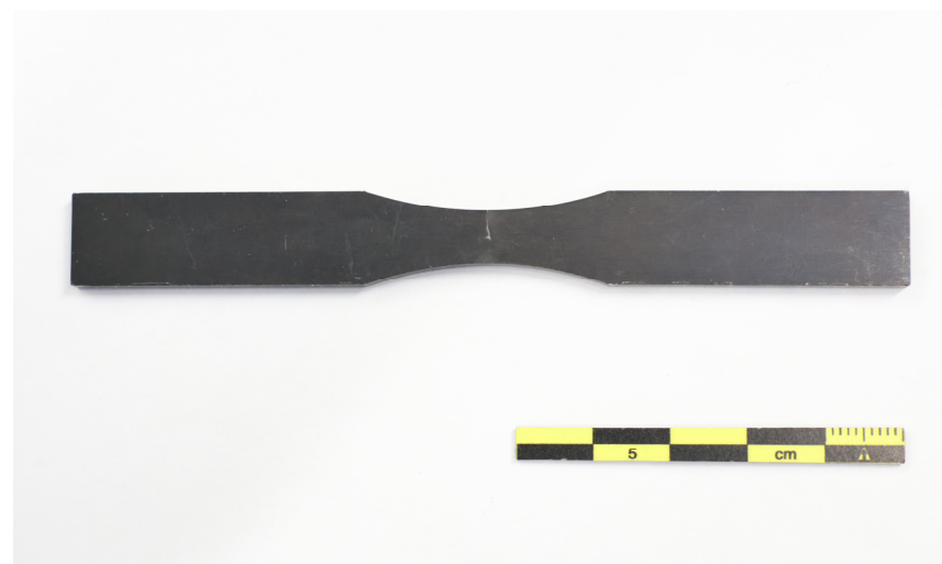
Figure 23. Oxidized sample after the breaking test.
