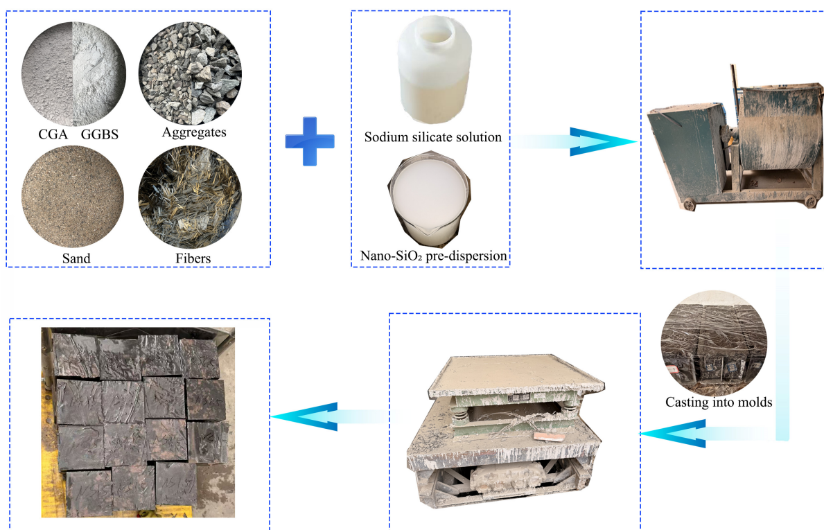
Figure 1. Preparation flow chart of specimens.
