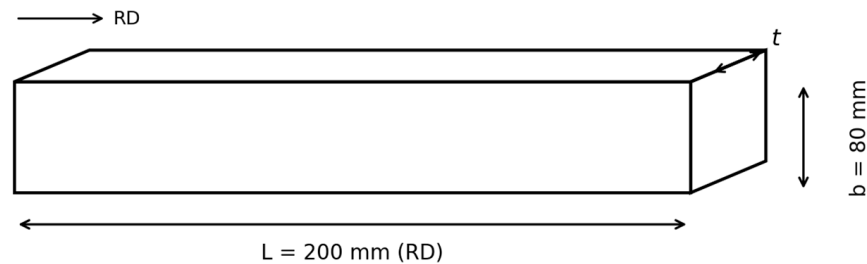
Figure 2. Geometry and dimensions of the rectangular four-point bending specimen.
