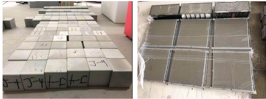
Figure 2. Cast concrete cube specimens before curing.
