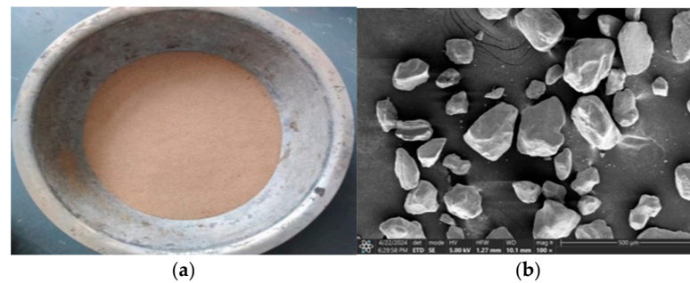
Figure 3. (a) Aeolian Sand, (b) SEM of Aeolian Sand.
