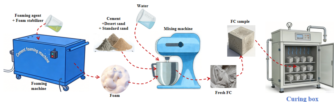
Figure 3. Preparation procedure of foam concrete (FC).
