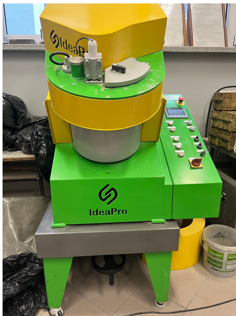
Figure 2. The machine used for artificial aggregate production.
