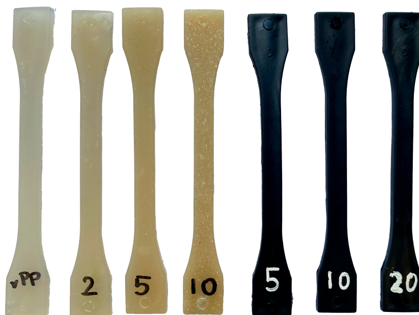
Figure 2. Injection-moulded dumbbell specimens of neat-recycled polypropylene (rPP) and rPP composites containing microcellulose fibres (MCFs, 2–10 pbw, left group) and microcellulose-derived biochar (BC, 5–20 pbw, right group).
