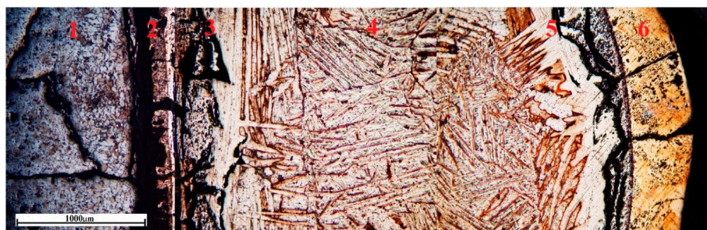
Figure 10. Change in the microstructure across the cross-section of a \text{CaTiO}_3/\text{VT1-0} alloy sample after isothermal interaction at 1720^\circ\text{C} for 430 s.
