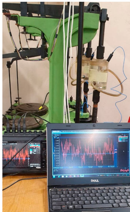
Figure 6. The measuring station for SCC at the constant tensile stress that can assess corrosion potential.
