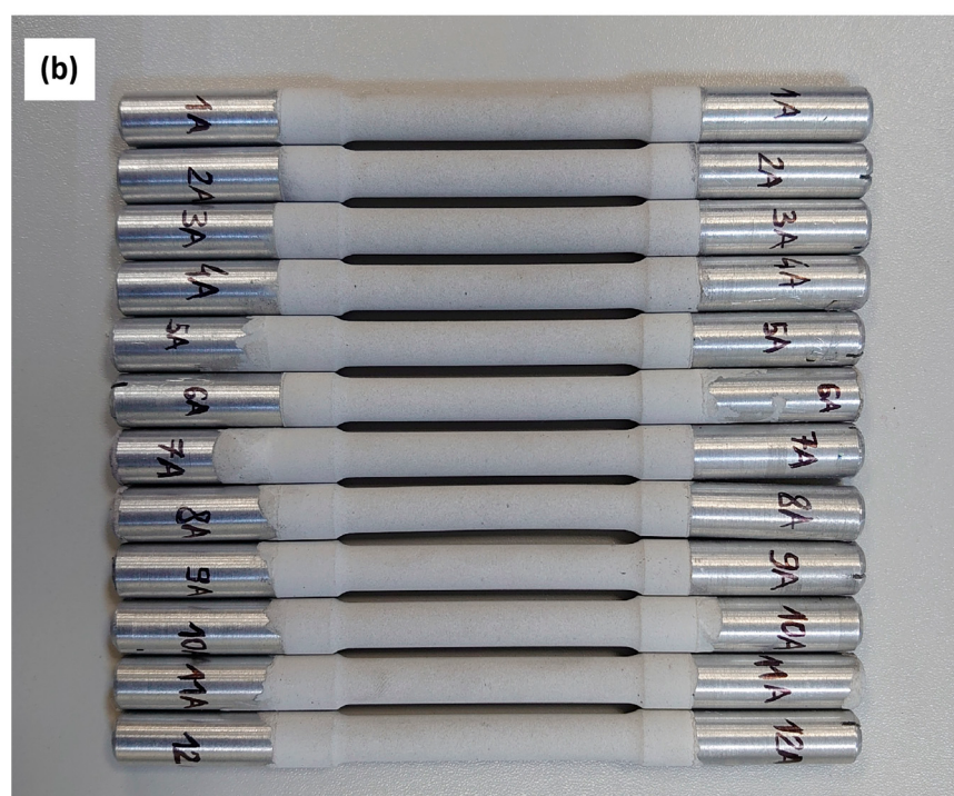
Figure 1. (a) Geometry and dimensions of the samples for tensile testing in accordance with PN-EN ISO 6892-1 standard L_0 = 50 mm, L_c = 70 mm, L_t = 165 mm, d_0 = 8 mm, S_0 = 50.27 mm 2 ( d_0 = 5 mm for the samples used in SCC testing with threaded grip sections—Figure 2); (b) A photo of the samples after PEO coating.
