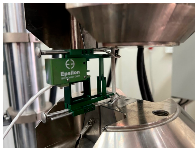
Figure 7. Al_2O_3 coated AW-5083 alloy sample after SCC testing in a universal testing machine with the extensometer Epsilon model 3542.
