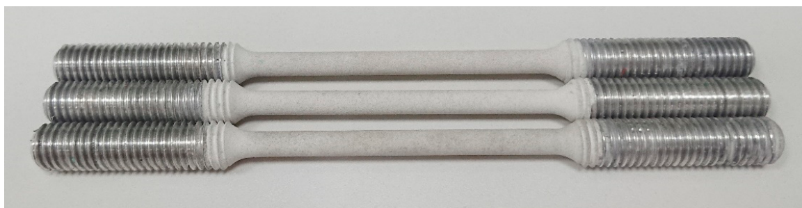
Figure 2. AW-5083 alloy samples with Al_2O_3 PEO coating and with threaded grip sections for SCC testing.
