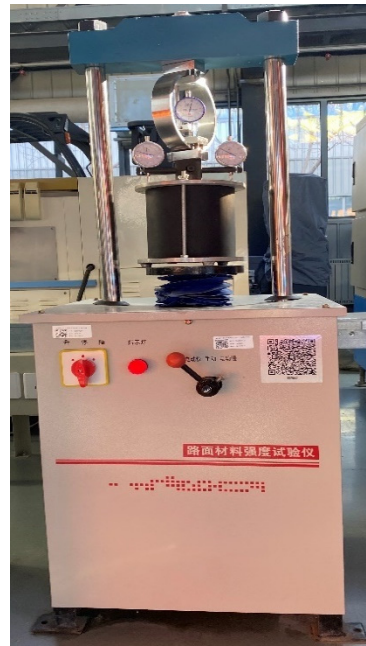
Figure 4. LD-127 pavement material strength tester.
