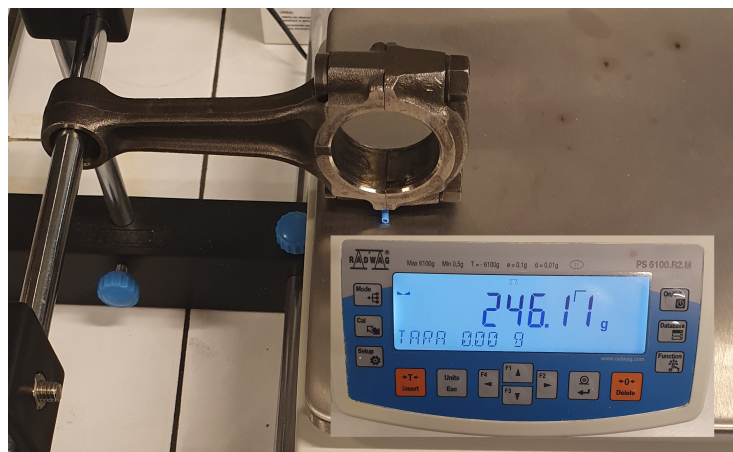
Figure 3. Weighing the connecting rod from a Suzuki GS650 engine, the weight indicates the fraction of the mass in rotation m_{c,B} = 0.24611 kg.
