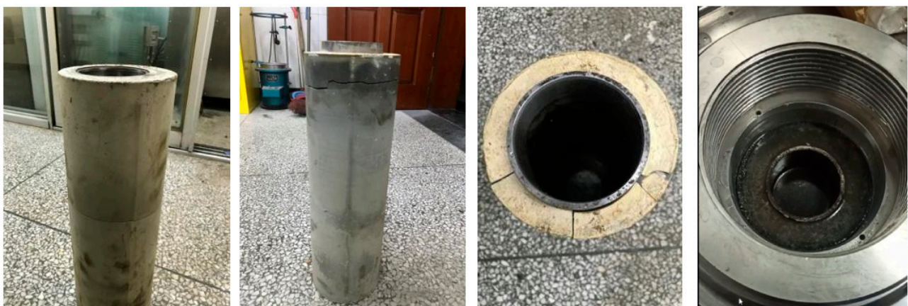
Figure 12. Cracking of cement annulus with blank formulation under 15 MPa cyclic pressure.
