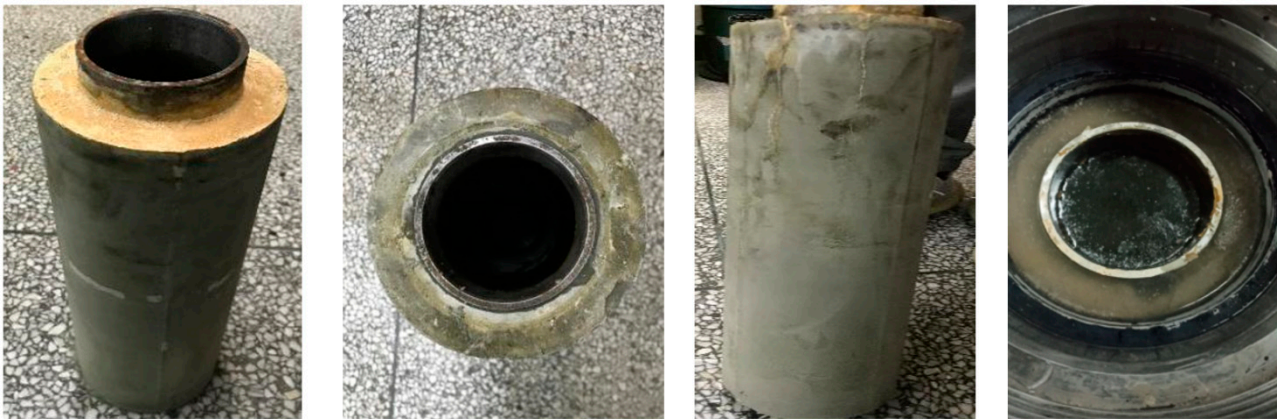
Figure 13. Integrity of cement annulus with toughened formulation under 30 MPa cyclic pressure.
