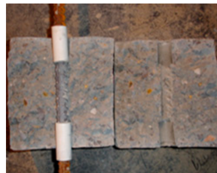
(b) Split into two pieces of damage
